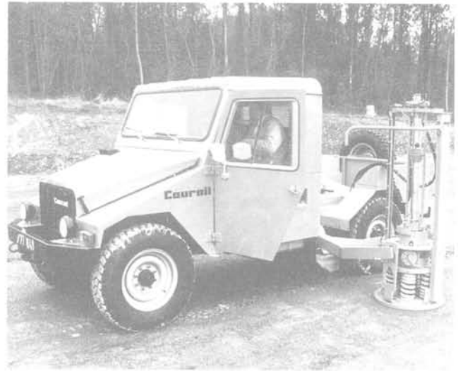
FIG. 10 Dynaplaque 1 (1982). Dynaplaque 1 test.
